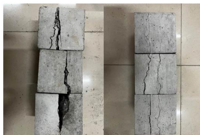
Figure 11. Concrete damage patterns
